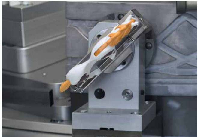
Jig with slotted link mechanism for printing on both sides of toys
