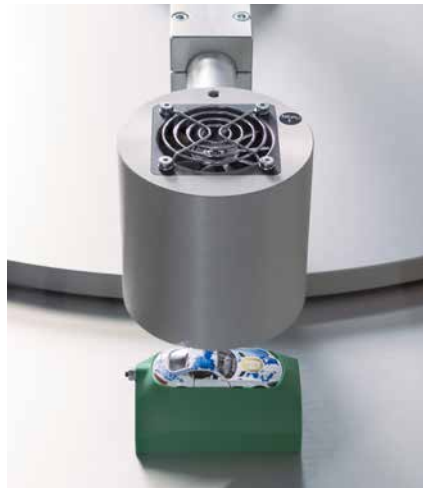
Component cold air drying – light surface drying of the pad printing ink for faster continuous printing
