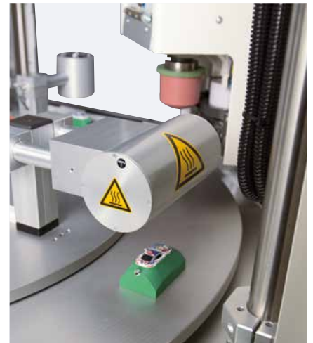
Component infrared-drying – shortens the drying time of the pad printing ink
