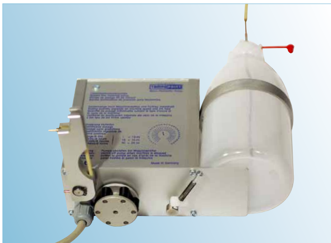
A. Connect flexible hose (1) with right and left connecting nipples (2 + 3) to the clamp ratchet (4).
