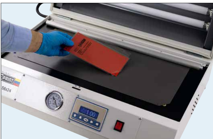
Cliché, film assembly plate and film are placed inside the exposure unit
