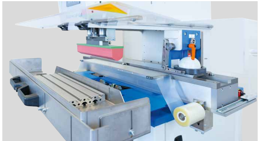
Standard drawer with integrated profile plate for workpiece insertion (left in picture)
